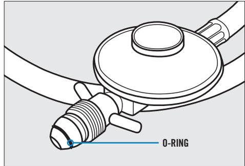
Figure 1: O-RING seal on the POL regulator.
